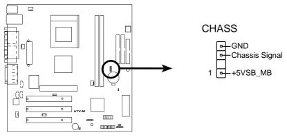
A7V-M Chassis Open Alarm Lead
